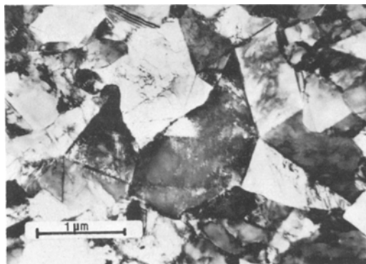
Fig. 3. Transmission electron micrograph of a nickel electrodeposit exhibiting a \langle 110 \rangle preferred orientation. Notice the five convergent twin planes in most of the grains.
